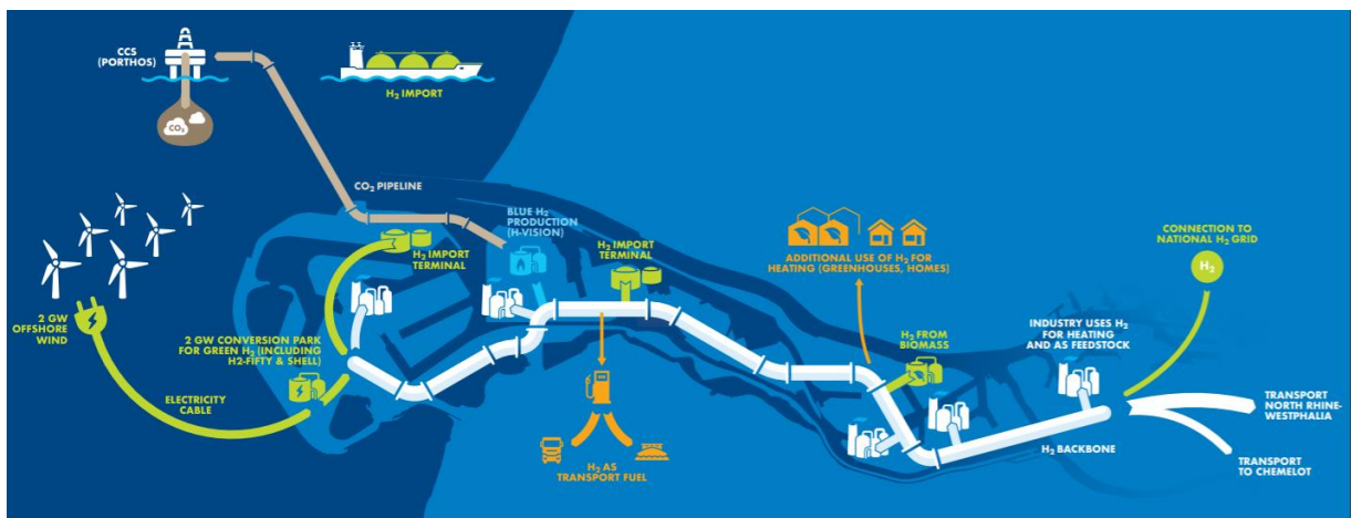
Figure 31: Regional hydrogen backbone port of Rotterdam combined with local production and import 113
