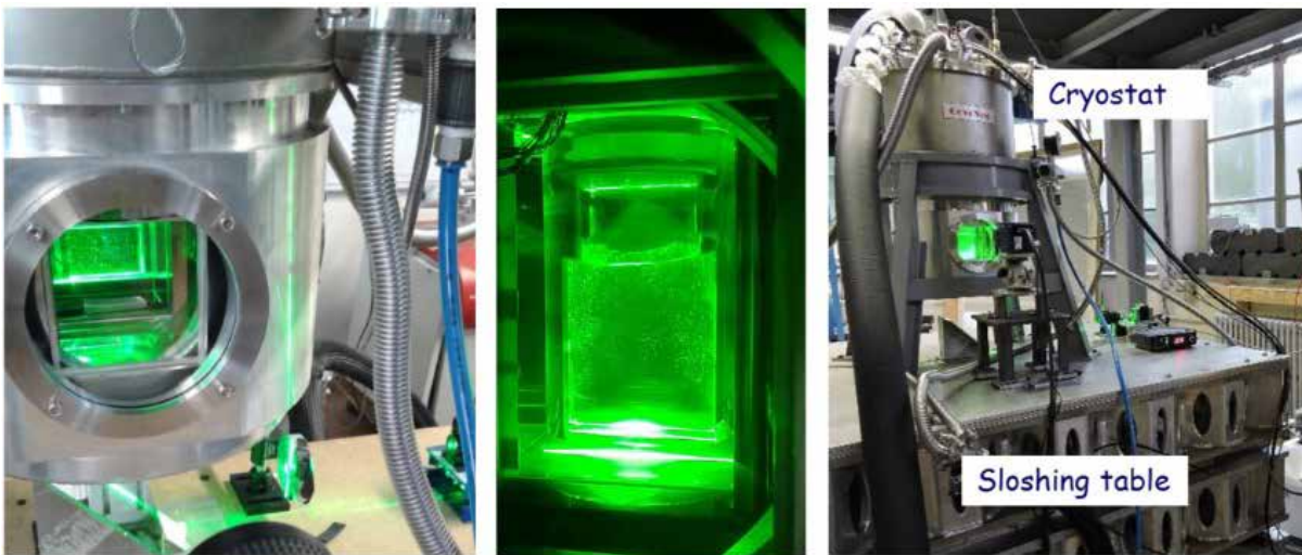
Experimental testing of sloshing of liquid hydrogen in a fuel tank, in the “Cryostat” test facility, with visualisation with Particle Image Velocimetry (PIV)
