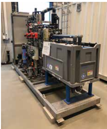
Electrodialysis reversal (EDR) pilot plant, capacity: 1.75 m 3 /d product water.
