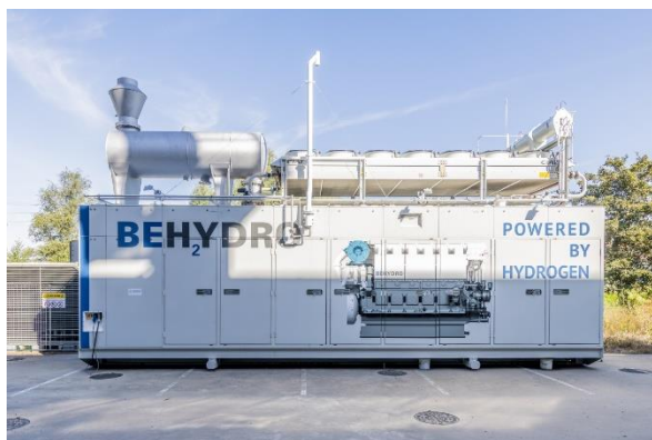
Figuur 16: 1 MW "dual fuel" genset van BeHydro
