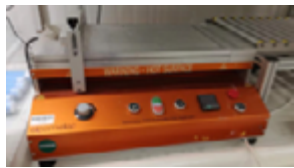
ELCOMETER 4340 Automatic Film Applicator • dimensions: 20/30cm • Heated coating bed
