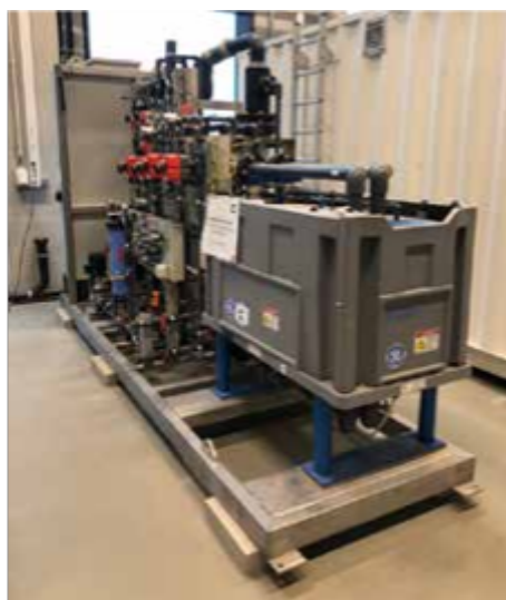
Figure 7: Electrodialysis reversal (EDR) pilot plant, capacity: 1.75 m 3 /d product water.
