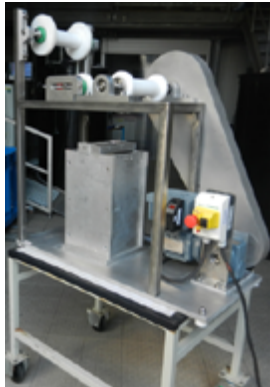
Roll-to-Roll Film Applicator • dimensions: 15cm width • speed: 1 to 800 cm/min
