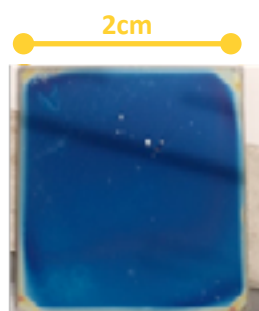
Photograph of thin-film photoactive cathode
