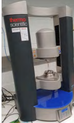
MODEL: HAAKE MARS™ 40 Rheometer □ Used to measure the viscosity of the slurry
