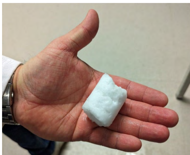
Figure 2: H 2 /CH 4 storage in clathrate hydrates
