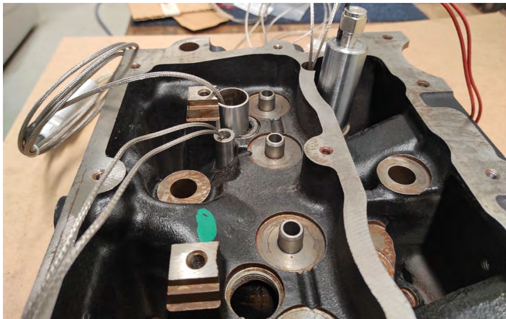
Modified engine cylinder head with instrumentation for direct measurement of surface temperature and wall heat flux (small cylinder near the centre of the image) as well as a prototype direct injector for hydrogen (large cylindrical object in the top right of the image)
